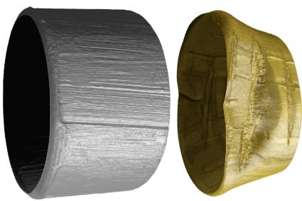
Bullet surface Deformed bullet surface
