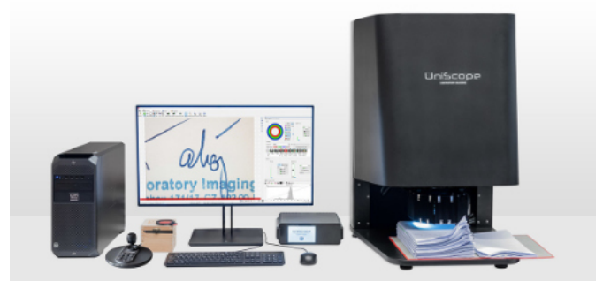
3D-scanning system with multispectral illumination.
