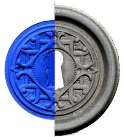
Split-line comparison of a silicone cast and the source object
