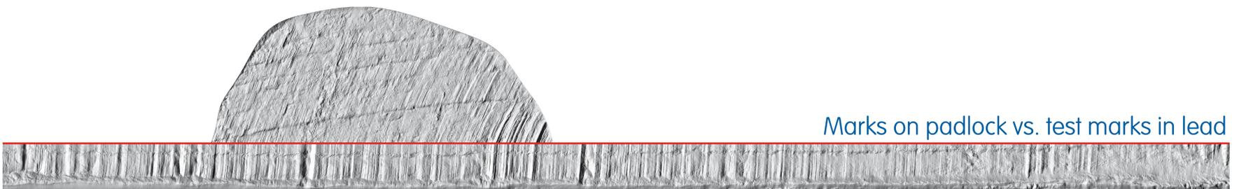
Marks on padlock vs. bolt cutter blade
